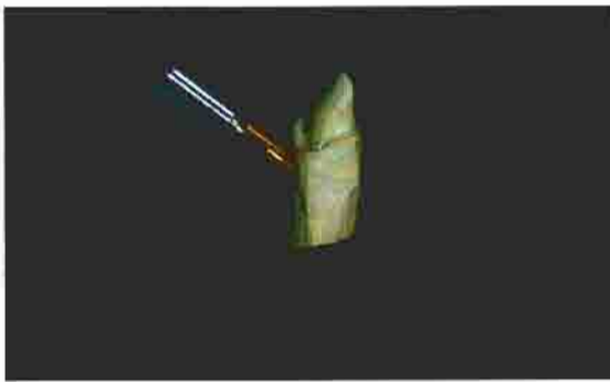
Figure 14 —A die fixed in the scanner with the contact digitizer preparing to digitize the die.
